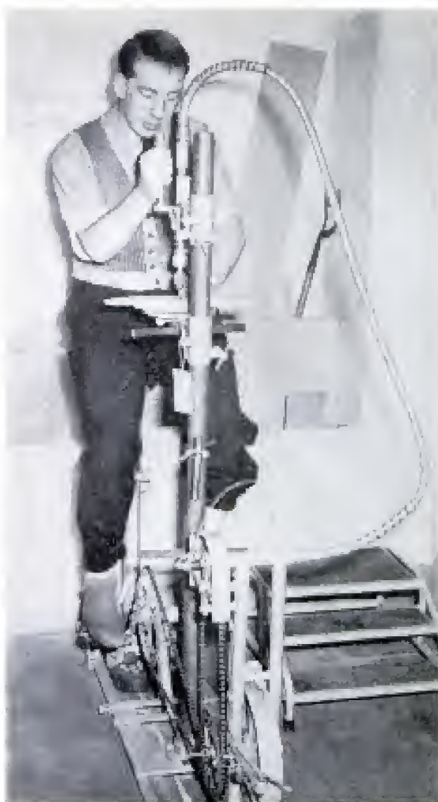
Using a pedal-driven drill operated through a flexible shaft, a patient gets work done and exercises weakened leg muscles. Below, slings brace weak arms and a press clamp grips bread while it is being cut
